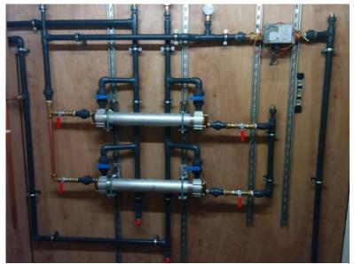
Figure 7: Shell and tube heat exchangers and the heat meter
