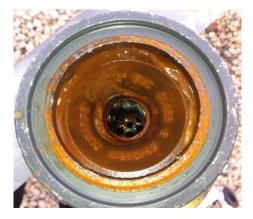
Figure 2: Heatexchanger after 2 years of run
